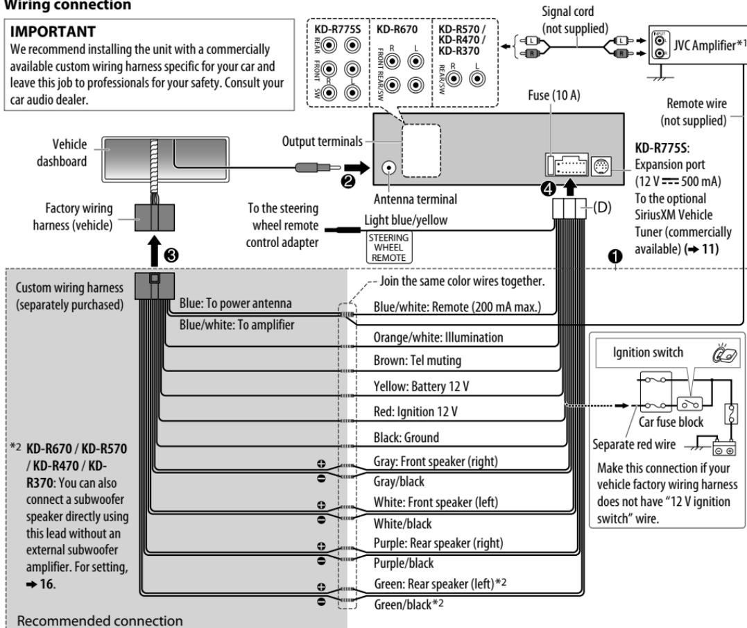
\*1 Firmly connect the ground wire of the amplifier to the car's chassis to avoid damaging the unit.
