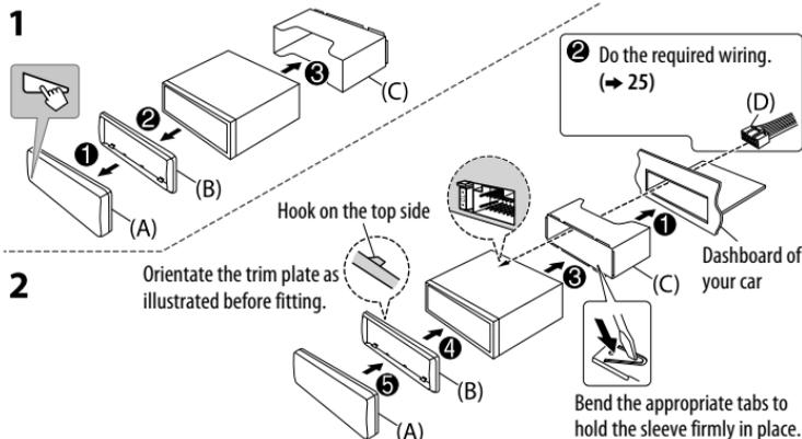
**When installing without the mounting sleeve**
